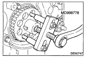
**■J** CRANKSHAFT SPROCKET "B" REMOVAL
