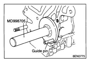
(4) Insert the installer aligning with the guide pin and install the bearing.
