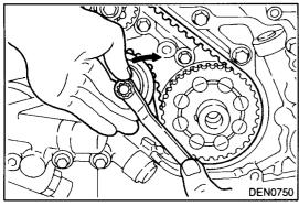
(4) More the tensioner "B" in the direction of arrow while lifting with a finger to give a sufficient tension to the tension side of the timing belt. In this condition, tighten the bolt to secure tensioner "B". When the bolt is tightened, use care to prevent the shaft from turning together. If the shaft is turned together, the belt will be overtensioned.
