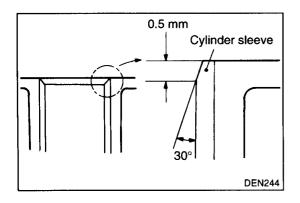
(5) Chamfer the cylinder sleeve top end as illustrated.
