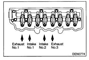
(2) Adjust the valve clearance at the points shown in the illustration.
