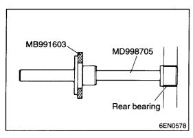
(3) Using the special tool, install the bearing.
