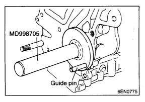
(5) Insert the installer aligning with the guide pin and install the bearing.
