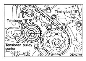
(3) Make sure that the pulley center and the bolt center are located as shown in the illustration.
