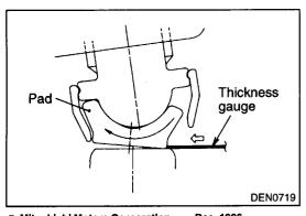
If an attempt is made to insert the thickness gauge without providing the clearance for it in advance by pushing the pad with a standard screwdriver or the like, the pad will tilt as shown in the illustration, preventing insertion of the thickness gauge.
