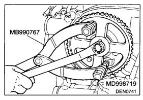
**◆B** CAMSHAFT SPROCKET BOLT LOOSENING
