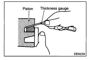
(2) In the case of semi-keystone type piston rings, check the ring to ring groove clearance as illustrated.
