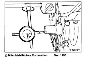
(8) After installing the bearing caps, make sure that the crankshaft turns smoothly and the end play is correct. If the end play exceeds the limit, replace the crankshaft bearings.
