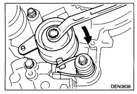
(2) Attach a bolt to the front end face of the timing belt tensioner. Fit an offset wrench onto the bolt and turn the wrench downward as shown to tighten the tensioner mounting bolt temporarily.
