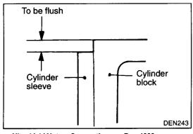
(4) Cut off the top end of the cylinder block in order to make the cylinder block flush with the sleeve. Cut off the minimum top end portion of the cylinder block necessary to make them flush. Do not cut off more than 0.2 mm.
