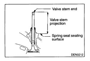
(2) Install the valve and, while pressing the valve against the valve seat, measure the valve stem projection between the valve stem end and the valve spring seat seating surface.
