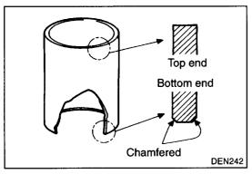
(3) Install with the chamfered end first as illustrated. Continue until the sleeve upper end is flush with the block upper end.
