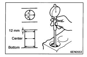
(3) Check the cylinder sleeve wall for scratches and seizure. If defects are evident, replace the cylinder sleeve. Measure the cylinder sleeve inner diameter at the points shown in the illustration. If it is badly worn, replace.
