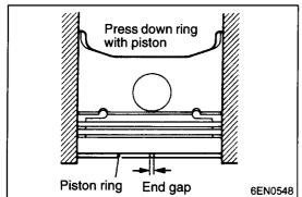
(3) Insert the piston ring into the cylinder bore. Force it down with a piston, its crown being in contact with the ring, to correctly position it at right angles to the cylinder wall. Then, measure the end gap with a thickness gauge. If the end gap is excessively, replace the piston ring.
