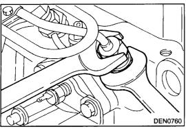
(2) When tightening the injection pipe nuts, hold the hexagon nut of the return pipe with a spanner in order to prevent it from rotating along with the nut.
