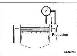
at any one location exceeds the protrusion tolerance shown for any rank in the following table, use the gasket one rank higher that rank.
