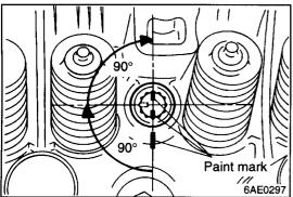
(3) Using the special tool (MB991654) and according to the tightening sequence, tighten the bolts to the specified torque.
