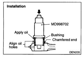
(2) Using the special tool, install the bushing, aligning the oil hole of the bushing with the oil hole at the small end of the connecting rod.
