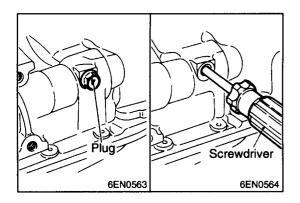
(4) Remove the plug on the cylinder block and insert a Phillips screwdriver [shank diameter 8 mm] through the hole. If it can be inserted as deep as 60 mm or more, the timing marks are correctly aligned. If the inserted depth is only 20 – 25 mm, turn the oil pump sprocket one turn and realign the timing marks. Then check to ensure that the screwdriver can be inserted 60 mm or more. Keep the screwdriver inserted until installation of the timing belt is finished.
